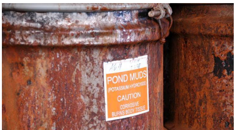
Corroded Drum of "KOH Mud" with Warning Label
